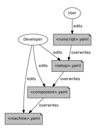
Fig. 1: ESM-Tools configuration files hierarchy
