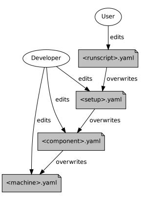
Fig. 1: ESM-Tools configuration files hierarchy
