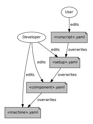
Fig. 1: ESM-Tools configuration files hierarchy
