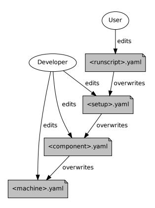
Fig. 1: ESM-Tools configuration files hierarchy
