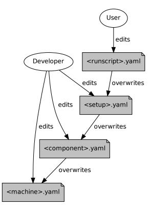
Fig. 1: ESM-Tools configuration files hierarchy
