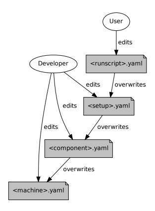
Fig. 1: ESM-Tools configuration files hierarchy
